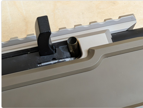
Spent case tipped sideways and jammed in the ejection port after firing.
