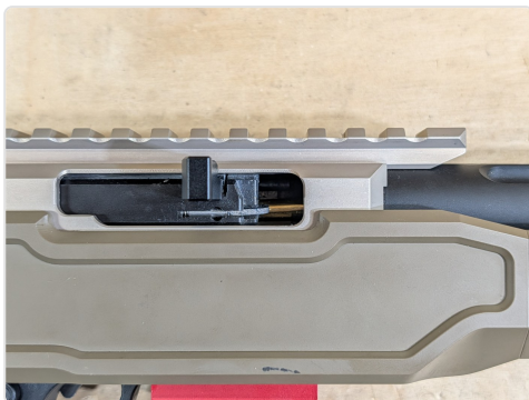
Round stopped partway into the chamber, bolt not fully forward.
