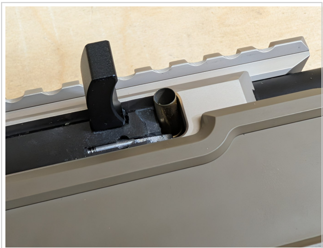
Spent case tipped sideways and jammed in the ejection port after firing.
